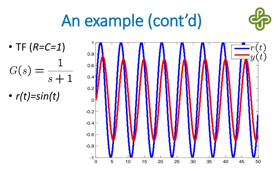
At steady-state, *r(t)* and *y(t)* has same frequency, but different amplitude and phase!
